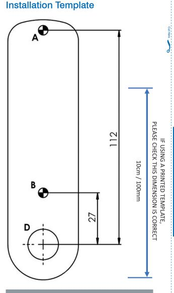
HOLES A, B & C DIAMETER 4.5 / 5.0mm HOLE D DIAMETER 16.5 / 17mm ALWAYS USE FIXING HOLE A and B
