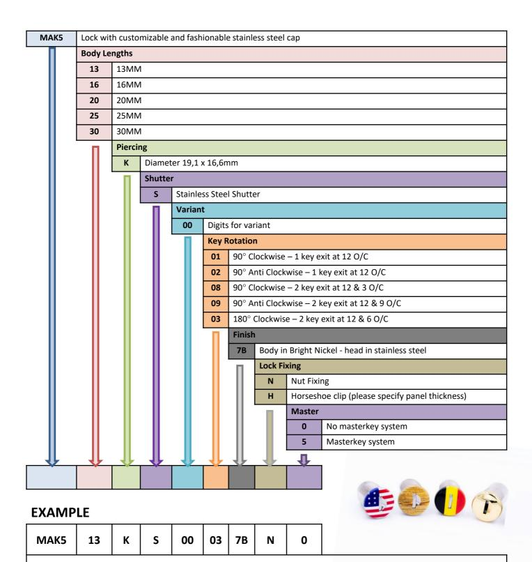
Lock with 13mm under the head - fixing hole size diameter 19,1 x 16,6mm - 180 $^{\circ}$  Movement Clockwise 2 key exits - nickel finish - Nut fixing — Without Master
