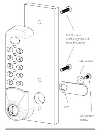
HOLES A, B & C DIAMETER 4.5 / 5.0mm HOLE D DIAMETER 16.0 / 16.5mm ALWAYS USE FIXING HOLE A AND USE EITHER FIXING HOLE B OR C. Recommended screw fixing torque 0.8Nm
