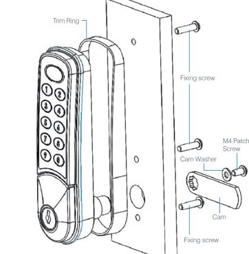
Remove battery pull tab before fixing lock
